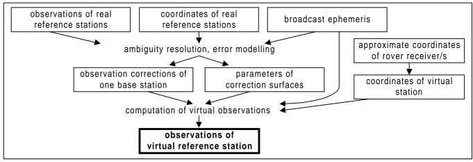
Fig. 2: Computation of carrier phase observations of a virtual reference station in a regional GPS-network.
