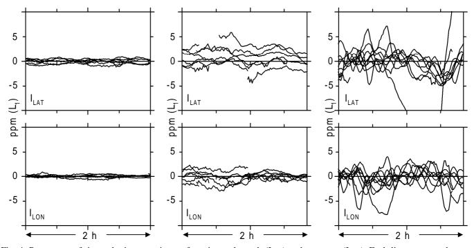
Fig. 4. Parameters of ionospheric correction surfaces in north-south ( $I_{LAT}$ ) and east-west ( $I_{LON}$ ). Each line connects the parameters of a single satellite. Left panels: low vertical electron content (VEC) <10<sup>10</sup> el/m<sup>2</sup>, no disturbances. Center panels: high VEC (40...50<sup>10</sup> el/m<sup>2</sup>), no disturbances. Right panels: low VEC (<15<sup>10</sup> l<sup>6</sup> el/m<sup>2</sup>), MSTIDs.
