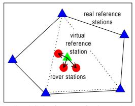
Fig. 1: Virtual GPS reference station in a regional network. The observations of the virtual station are computed from the observations of three or more real reference stations.
