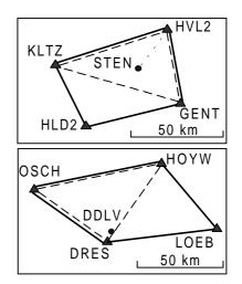
Fig. 7. Two sub-networks with reference station distances of about 60 km.
