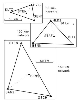
Fig. 8. Three sub-networks with reference station distances of about 60 km, 100 km and 150 km.
