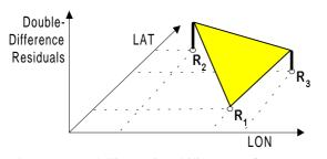
Fig. 3. Error modelling using bilinear surfaces are depicted best for double differenced observables. The actual algorithm is based on undifferenced observables.
